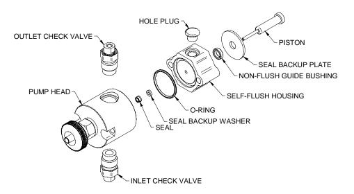
Figure 5-2. Stainless Steel Non-Self-Flushing Pump Head Assembly
